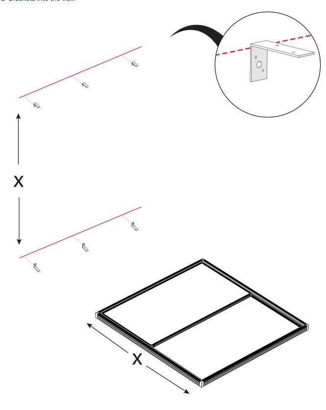
Carefully lift the markerboard assembly and set onto the brackets.
