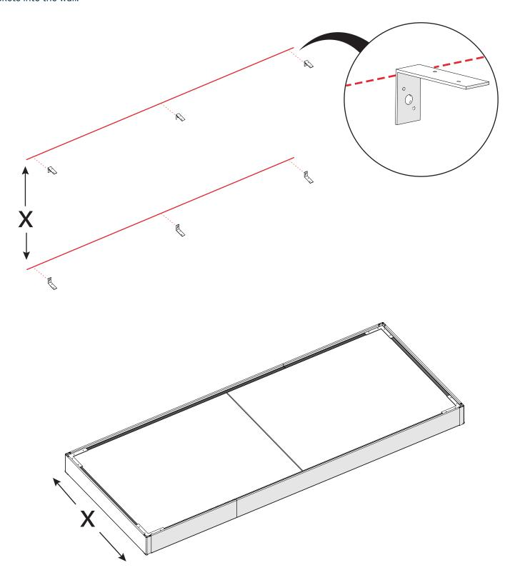
Carefully lift the markerboard assembly and set onto the brackets.
