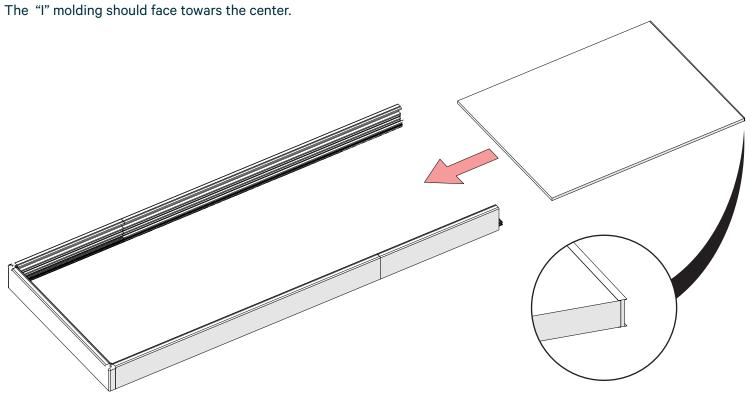
Slide the second board through the channel. The inside will fit into the "I" molding.
